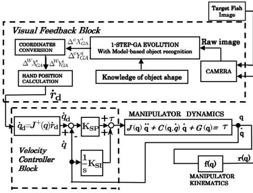
Fig. 1. Block diagram of the control system
