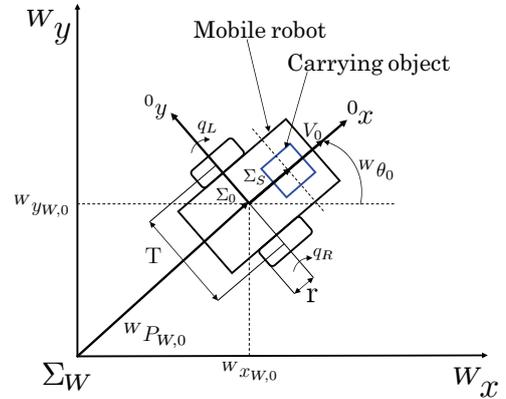
Fig. 1. Mobile robot on the standard of coordinates
