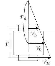
Fig. 4. Relation between  $r_c(t)$  and velocity of wheels
