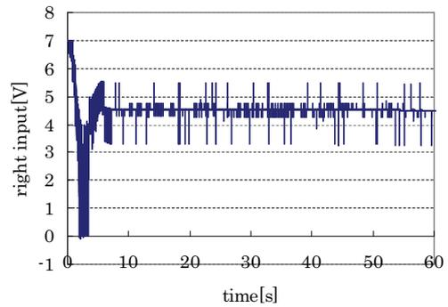
Fig. 15 Right input voltage when PID control applies
