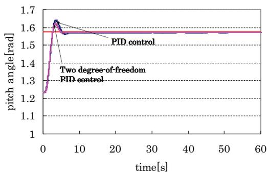
Fig. 12 Comparison of pitch angle
