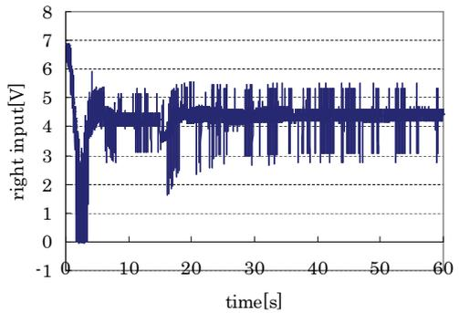
Fig. 22 Right input voltage when two degree-of-freedom PID control applies
