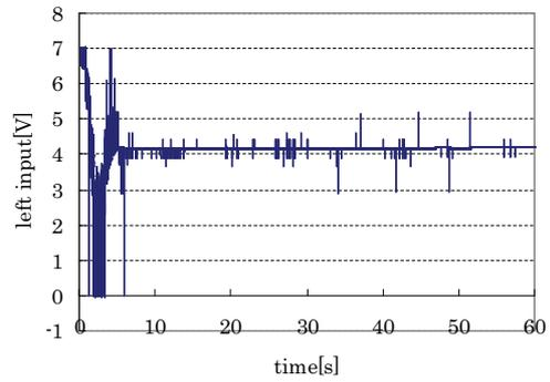
Fig. 14 Left input voltage when two degree-of-freedom PID control applies
