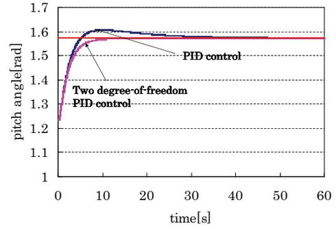
Fig. 5 Comparison of pitch angle
