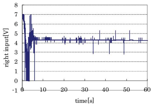
Fig. 16 Right input voltage when two degree-of-freedom PID control applies
