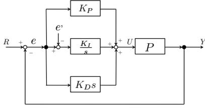
Fig. 4 Two degree-of-freedom PID control structure
