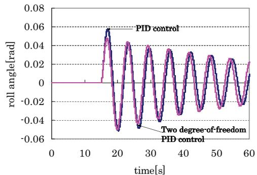
Fig. 8 Comparison of roll angle
