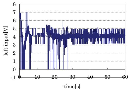
Fig. 19 Left input voltage when PID control applies
