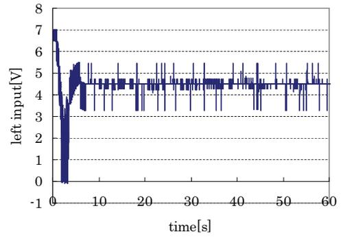
Fig. 13 Left input voltage when PID control applies
