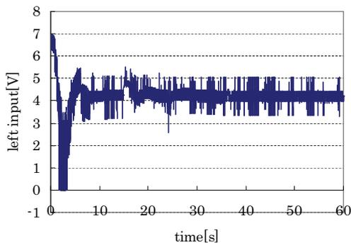
Fig. 20 Left input voltage when two degree-of-freedom PID control applies
