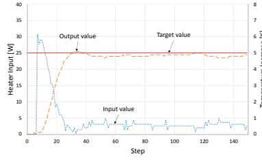
Fig. 7. GPC Experiment Result for Tuned Parameters
