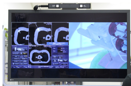
図 7 Monitor displaying both of CT image and tip of needle
