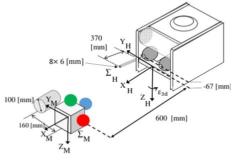
Fig.13 Docking coordinate system.
