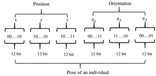
**Fig.5** An individual of GA population: 12 bits for each  $x$ ,  $y$ ,  $z$  represents the position coordinate of the three dimensional model of the gene and 12 bits for each  $\epsilon_1$ ,  $\epsilon_2$ ,  $\epsilon_3$  describes the orientation defined by a quaternion.
