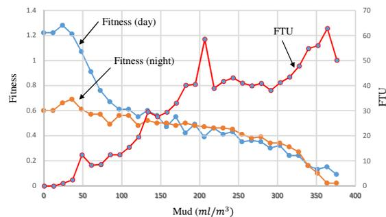
Fig.9 Fitness values against turbidity at the distance 600 mm between the ROV and 3D marker. The fitness value is nearly same in day and night time above 30 FTU.
