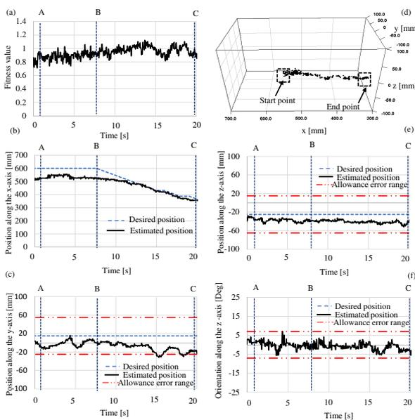
**Fig.11** Docking performance against turbidity (40 FTU) in the case of mud using dual-eye images recognition at 1280 Lx (maximum lighting condition): (a) fitness value, (b) position along the x-axis, (c) position along the y-axis, (d) 3D trajectory of the underwater vehicle, (e) position along the z-axis, and (f) orientation along the z-axis.
