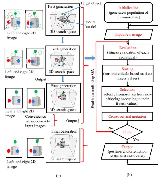
**Fig.6** Flowchart of the real-time multi-step GA: (a) the recognition process of the target pose is evaluated in 2D, convergence occurs in 3D (b) the flowchart of the RM-GA, the best solution is evaluated within 33 ms through the GA process.
