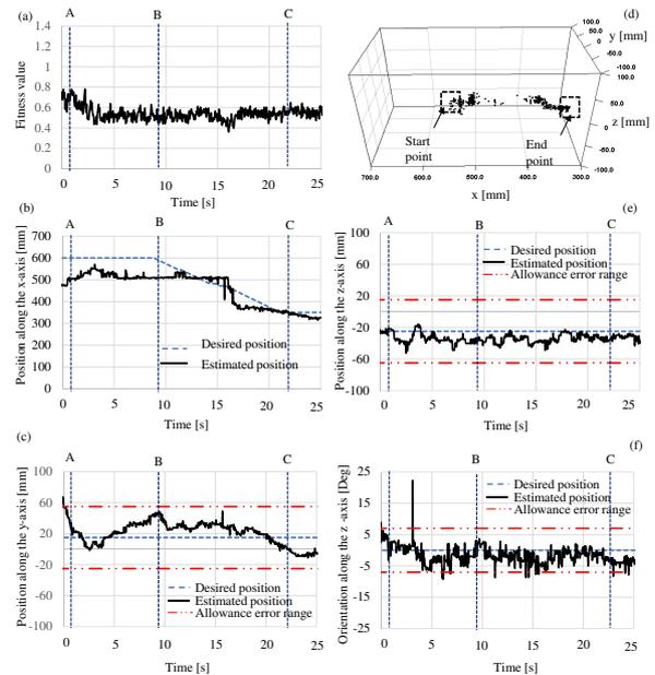
**Fig.12** Docking performance against turbidity (40 FTU) in the case of mud using dual-eye images recognition at 80 Lx (minimum lighting condition): (a) fitness value, (b) position along the x-axis, (c) position along the y-axis, (d) 3D trajectory of the underwater vehicle, (e) position along the z-axis, and (f) orientation along the z-axis.
