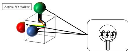
Fig.8 Active 3D marker: Red, green and blue LED were installed into the white spherical ball and covered by colour balloon.
