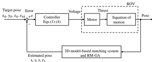
Fig.7 Block Diagram of Visual Servo Control.
