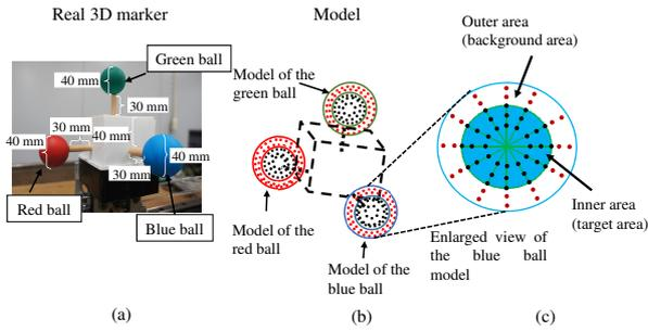
**Fig.4** Real 3D marker and model: (a) real 3D marker, (b) model, (c) enlarged view of the blue ball model, where the inner area is the same size as the real target object (blue ball) and the outer area is the background area. The dots in (c) mean points to calculate the correlation degree on how much the inner area overlaps the blue ball and the outer area does not overlap the blue ball.
