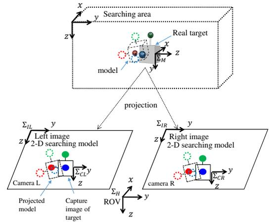
Fig.2 Model-based matching method using dual-eye cameras and 3D marker
