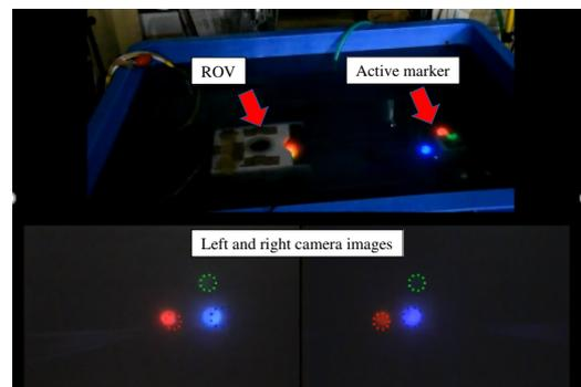
**Fig.1** Docking experiment in turbid water using an active marker under changing lighting environment.
