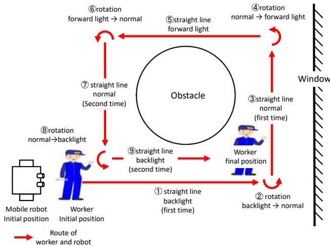
Fig. 12. The route of the tracking experiment
