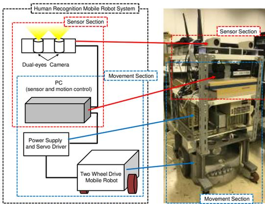
Fig. 1. Human Recognition Mobile Robot System up to 0.6 [m/s].
