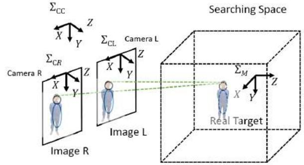
Fig. 6. Model-based Matching System using Dual-eyes Vision System
