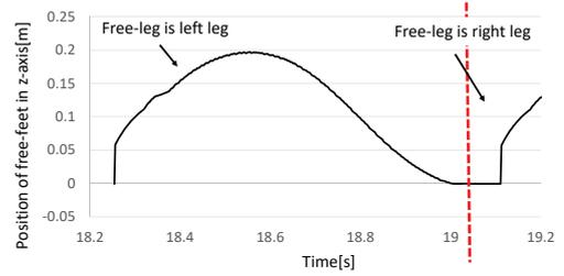
Fig. 6. Z-Position of free-leg in one step
