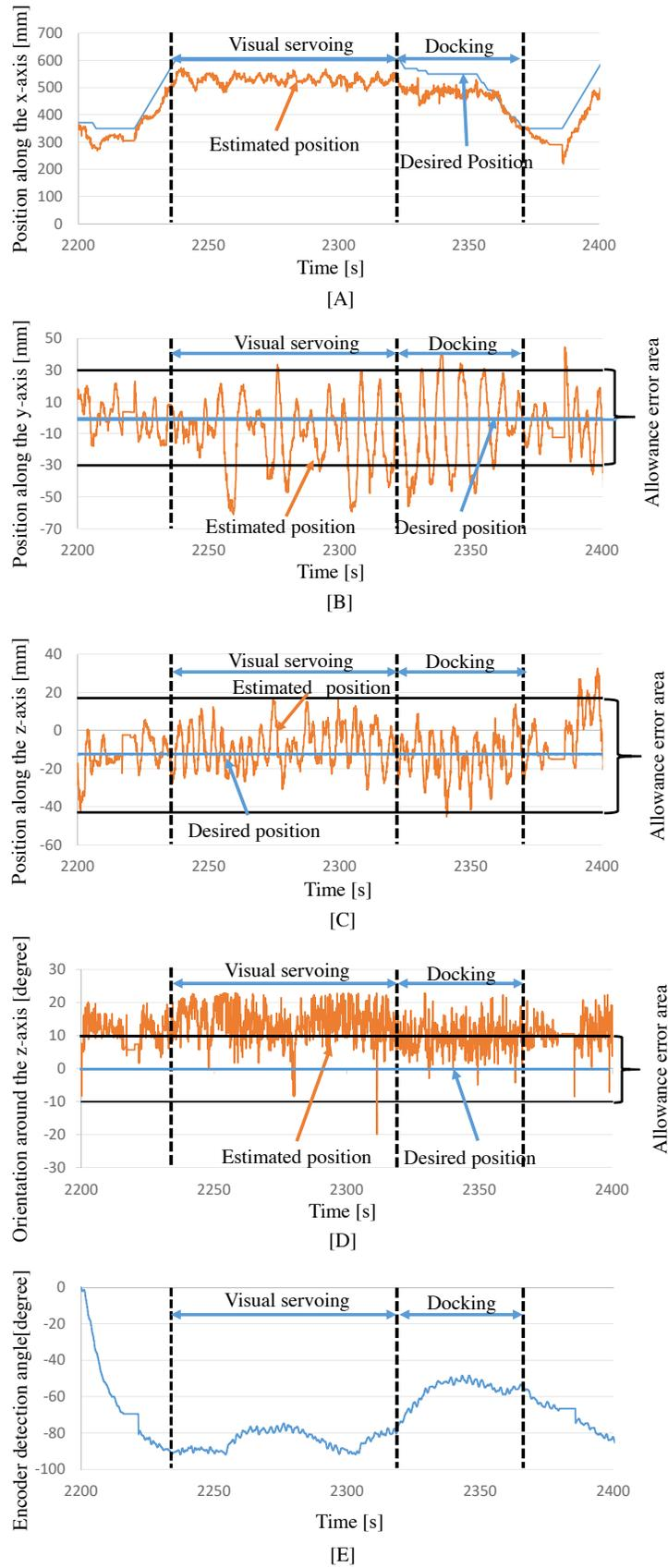
Fig. 12. Docking Result Against The Rotary Station: (A) Position along The X-axis, (B) Position along The Y-axis, (C) Position along The Z-axis, (D) Orientation around The Z-axis, (E) The Encoder detects Angle
