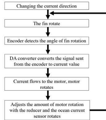
Fig. 4. Flowchart of an autonomous rotary docking station
