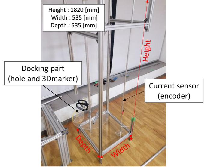
Fig. 8. The Autonomous Rotary Station for Pool
