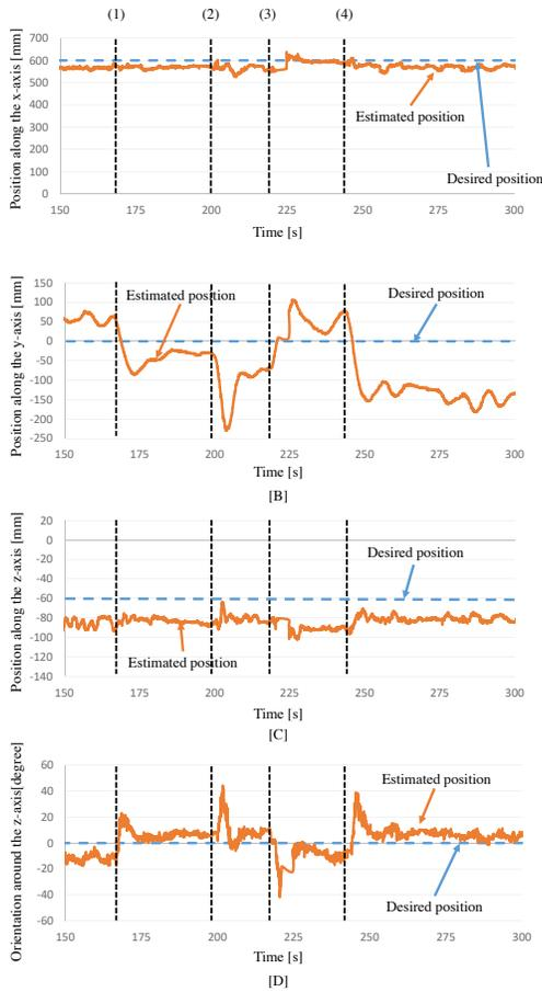
Fig. 10. Experimental result of VS against the autonomous rotary station.
