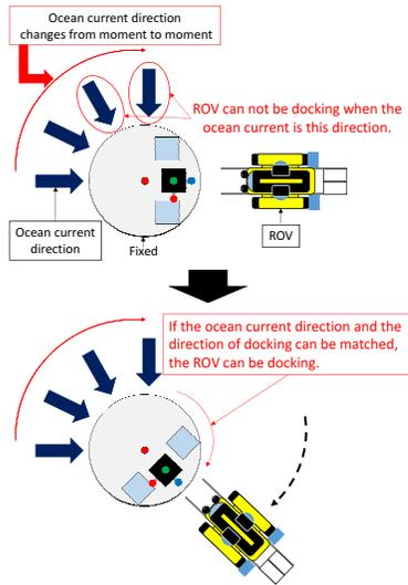
Fig. 1. Operation image of an autonomous rotary station
