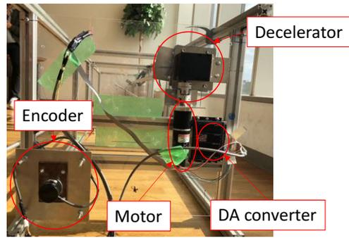
Fig. 3. Structure at the top of an autonomous rotary station
