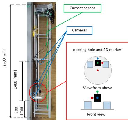
Fig. 2. Overall view of an autonomous rotary station
