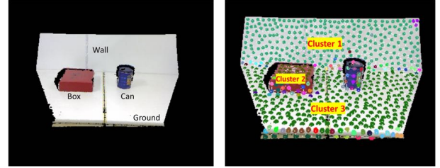
Fig.4 Input data. (a) Original 3D point cloud data. (b) Result of GNG-DT.
