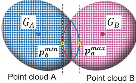
Fig. 7. Condition occurring contact
