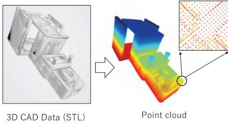
**Fig. 3.** Conversion of data from STL to point cloud
