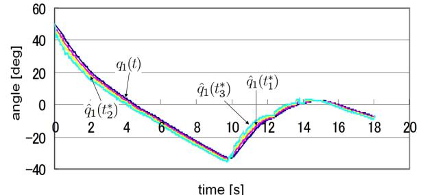
Fig. 16. Actual and predictive angle of link 1 ( $\tilde{t}=0.15$ [s])
