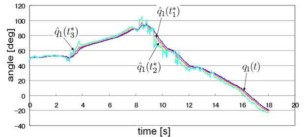
Fig. 21. Actual and predictive angle of link 1 ( $\tilde{t}=0.15[\text{s}]$ )
