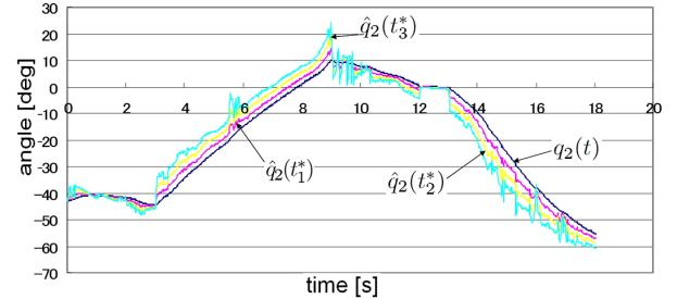
Fig. 20. Actual and predictive angle of link 2 ( $\tilde{t}=0.3[\text{s}]$ )
