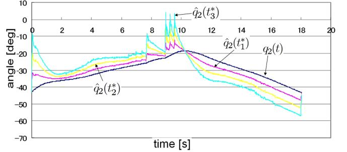
Fig. 8. Actual and predictive angle of link 2 ( $\tilde{t}=1.2[\text{s}]$ )
