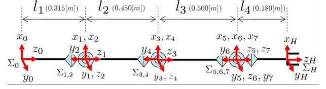
Fig. 5. Coordinate system of PA10
