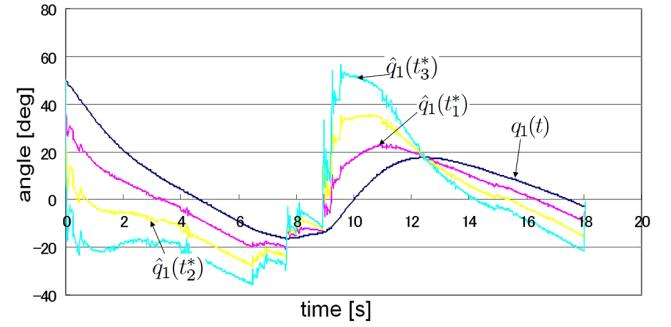
Fig. 7. Actual and predictive angle of link 1 ( $\tilde{t}=1.2[\text{s}]$ )
