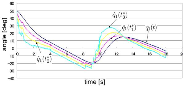
Fig. 12. Actual and predictive angle of link 1 ( $\tilde{t}=0.6$ [s])
