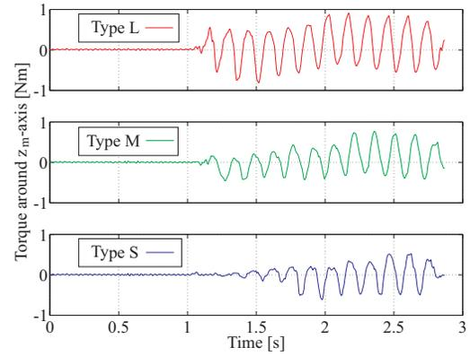
Fig. 5. Measured reaction torque around the  $z_m$ -axis in the successful state
