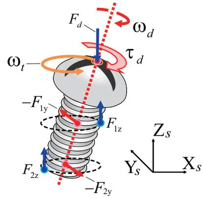
Fig. 9. Force and torque acting on the external thread
