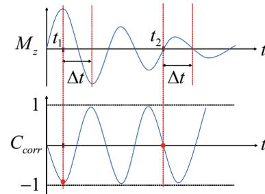
Fig. 14. Calculation example of the coefficient of autocorrelation
