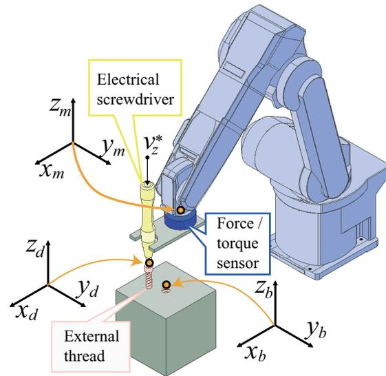
Fig. 1. Robot system configuration for thread fastening task
