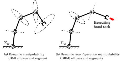
Fig. 2 (a) Dynamic manipulability ellipsoids (DMEs), (b) dynamic reconfiguration manipulability ellipsoids (DRMEs)
