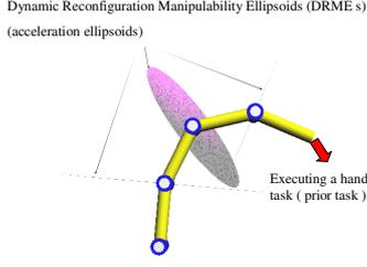
Fig. 1 Application of Dynamic Reconfiguration Manipulability for redundant manipulator
