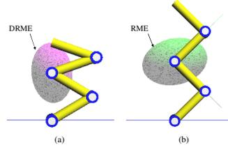
Fig. 4 Shapes of manipulator: (a) shape of the peak of 2nd-link's DRMM with DRME, (b) shape of the peak of 2nd-link's RMM with RME
