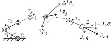
Fig. 3 Reconfiguration at intermediate link during hand task executed
