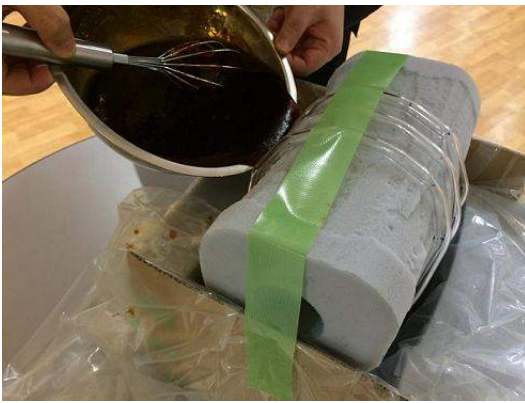
Fig. 11. Making skin of CT-IVR phantom
