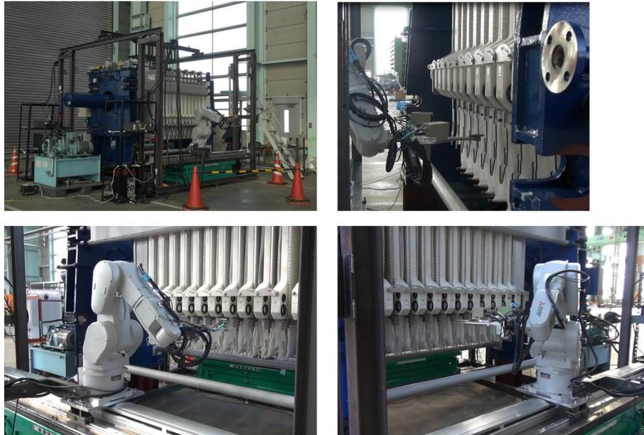
Fig. 1 Robot system for removing filter clothes of filter press machine.
