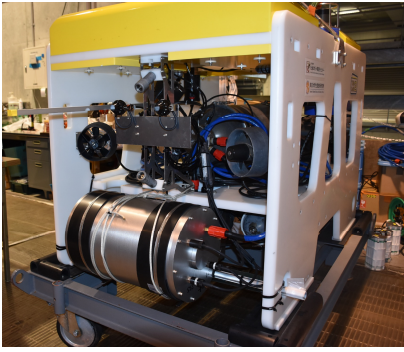
Fig. 5. Photo of Tuna-Sand 2 with GA PC and dual-eye camera
