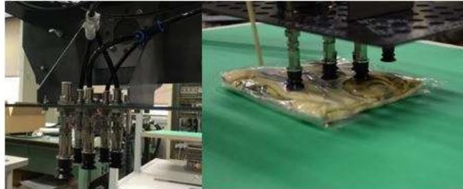
Fig. 21 Four absorption pads under robot hand
