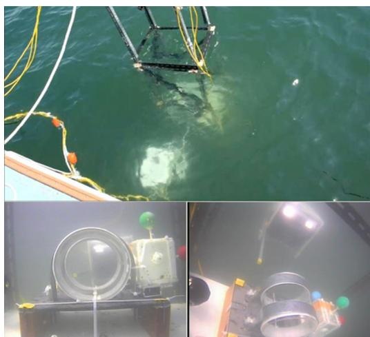
**Fig. 28** Continuous iterative docking experiments in the sea. These photographs were taken by two underwater cameras installed in the docking station and from a pier
