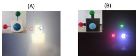
Fig.3 Image of 3D Marker Viewed from ROV Camera. (A)Passive 3D Marker (B)Light Emitting 3D Marker
